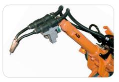
KempArc Pulse TCS can be delivered with a welding torch option of your choice, either normal or push-pull model.
