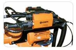
DT 400 wire feeders are equipped with the reliable 4-roll DuraTorque wire feeding mechanism and full metal feed rolls with excellent wear resistance.
