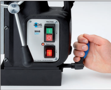
Release the adjustment feature
