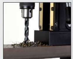
Twist drilling up to \varnothing 31.75 mm
