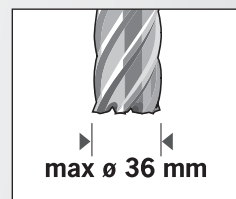
Core drilling up to ø 35 mm
