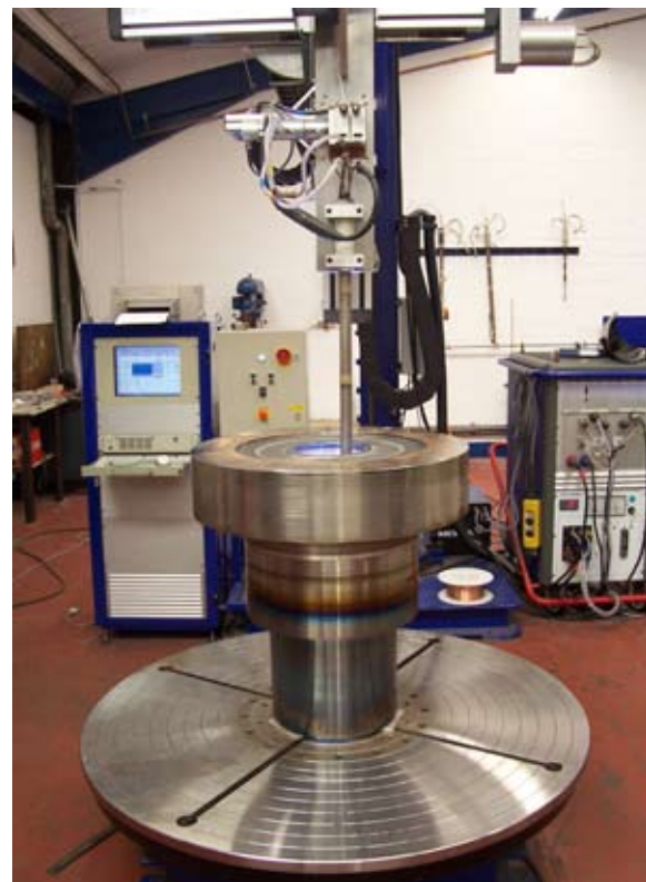
Mechanized welding equipment designed as fixed installation in the workshop. Cladding of the inside of workpieces with nickel base alloy.
