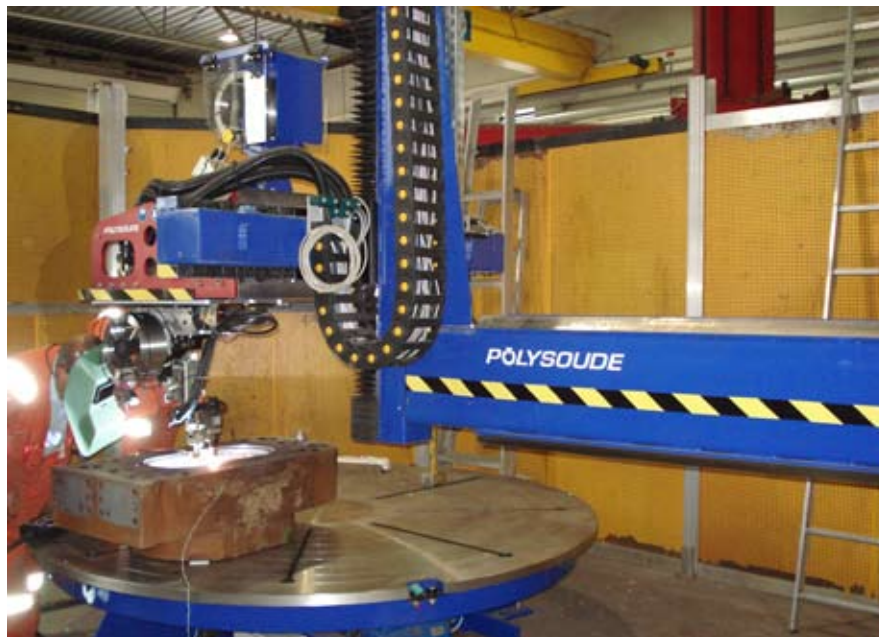
Unlimited number of rotations and move combinations between collector welding head at the column & boom enabling cladding operations of unusual geometries.
