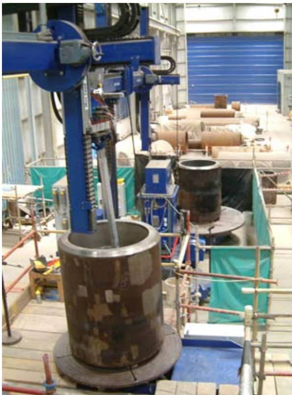
Mechanized welding equipment designed as fixed installation in the workshop. Cladding of the inside of workpieces with nickel base alloy.
