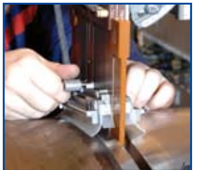
Torch module "Narrow Gap" for wall thicknesses up to 250 mm and more
