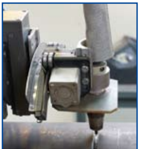
Torch module "MIG/MAG" with motorised torch inclination
