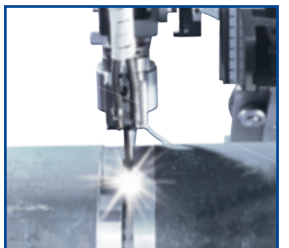
Torch module "V2 Narrow Gap" for wall thicknesses up to 75 mm
