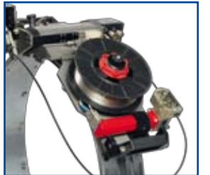
On-board wire feeder with straightening device
