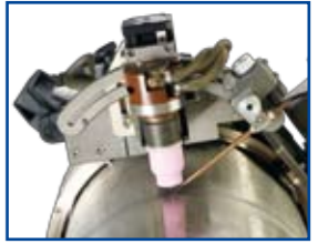
Torch block with AVC/OSC cross slides and adjustable wire guide
