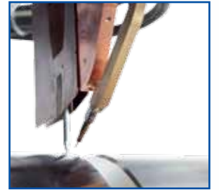
"Narrow Gap" torch with wire guide and integrated camera
