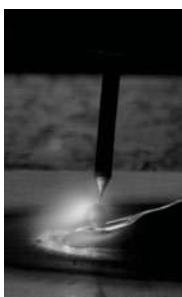
Droplet detachment after the pulse phase
