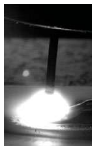
Droplet formation in the pulse phase
