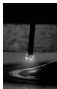
Cleaning and warm-up of the wire in the negative phase
