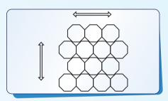
Each disc touches the adjacent curved surface. Primarily used where material flow is in all directions
