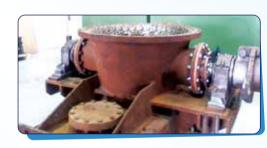
Final drive casing protected by to combat wear from primary material trapped between the housing and drive sprocket. Discs application was easy, due to the reduced amount of welding and minimal heat input causing no cracking in the housing.
