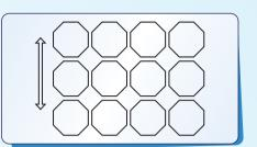
Discs touching at curved edge. Rows parallel and 10 mm part. Used where material flow is in direction of the arrow.
