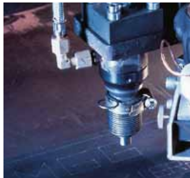
The optional high frequency punch marker permits accurate marking of points and lines.
