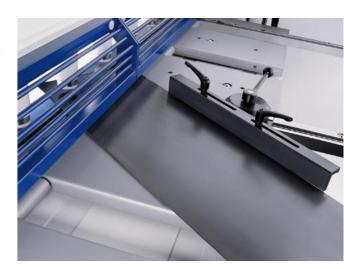
Reverse cutting with the stop aid The good parts leave the machine not at the rear but at the front. And that's the way it works: A swivel front gauge is mounted in the T-groove of the support bracket which then serves as front gauge.
