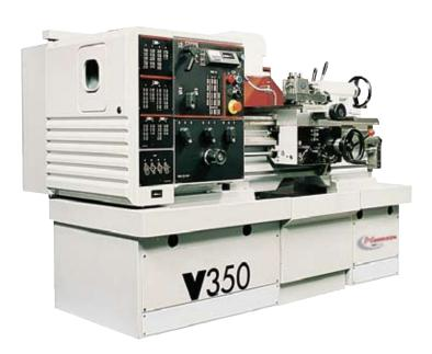
The V350's cast iron base provides maximum support for the torsionally stiffened bed and prevents swarf accumulation. The bed is epoxy resin bonded to the base and provides excellent structural damping and resistance to vibration.
