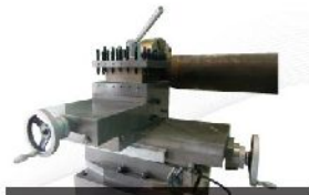
Cross and Longitudinal Compound Rest. (X1 and Z1 axes travel capability)
