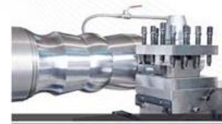
Hydraulic Copy Device (Templates are made by customers)
