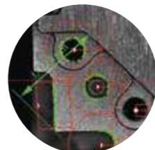
Erosion diameter measurement.
