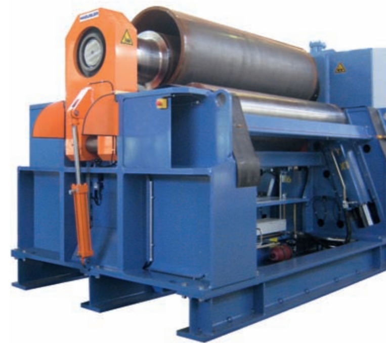
4-roller plate bending machine Type VRM-hy 3 000-610 Max. sheet width: 3 000 mm Max. wall thickness: 80 mm
