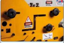
• Angle Station Cropping angle iron is possible for every angle between 45° and 90°, both internal and external.
