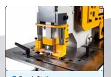
Punch Station The easy tool change system and swingaway stripper with fast manual adjustment assures a quick setup and is designed for a wide range of punching applications.
