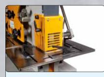
• Notching Station This versatile station is standard equipped with a rectangular notch unit. The notch table has adjustable back and side stops. Side notch applications are also possible.
