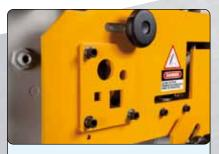
• Section Cutting Station The machines are fitted as standard with blades for cutting round and square bars. With extra equipment in this aperture, the machines are able to cut channel, beams or joist, T-section and many other special profiles.
