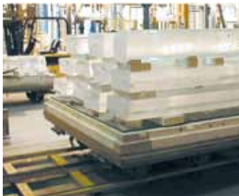
Bogie hearth furnace for tempering quartz rods
