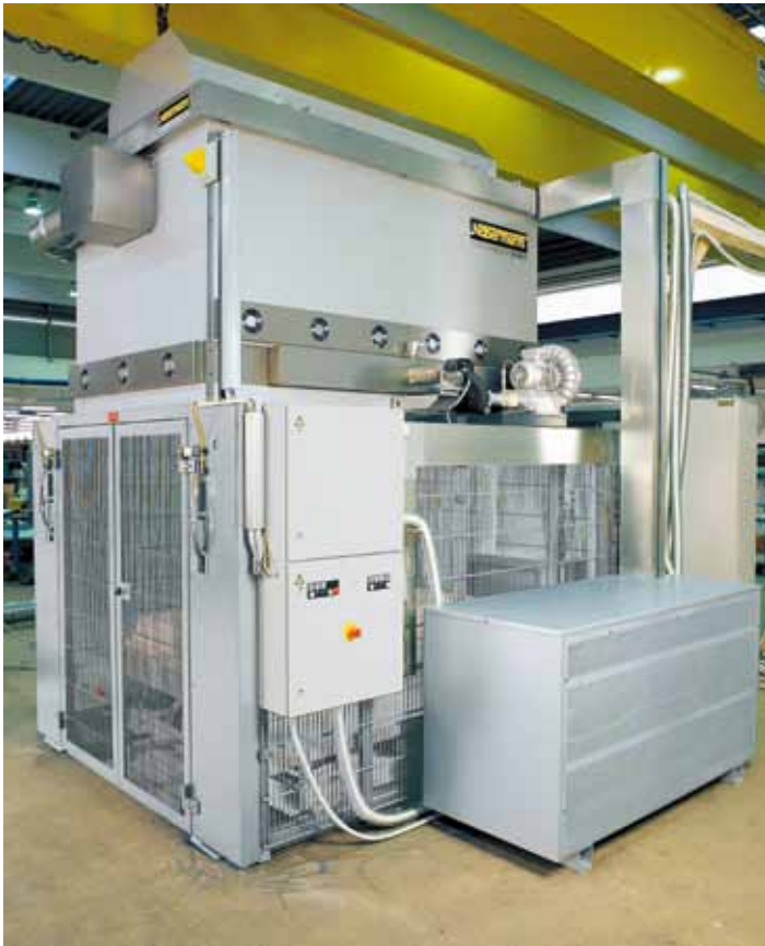
Combi high-temperature plants HT 1440/17 LBS with catalytic afterburning system for debinding and sintering in one process
