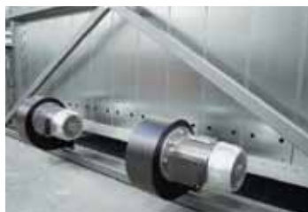
Indirect cooling behind the insulation for reduction of turbulences in the furnace chamber
