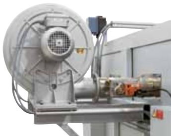
Cooling fan for accelerated cooling
