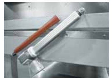
Automatic lid opening via electromechanical spindle
