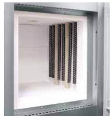
Vertically mounted SiC rods
