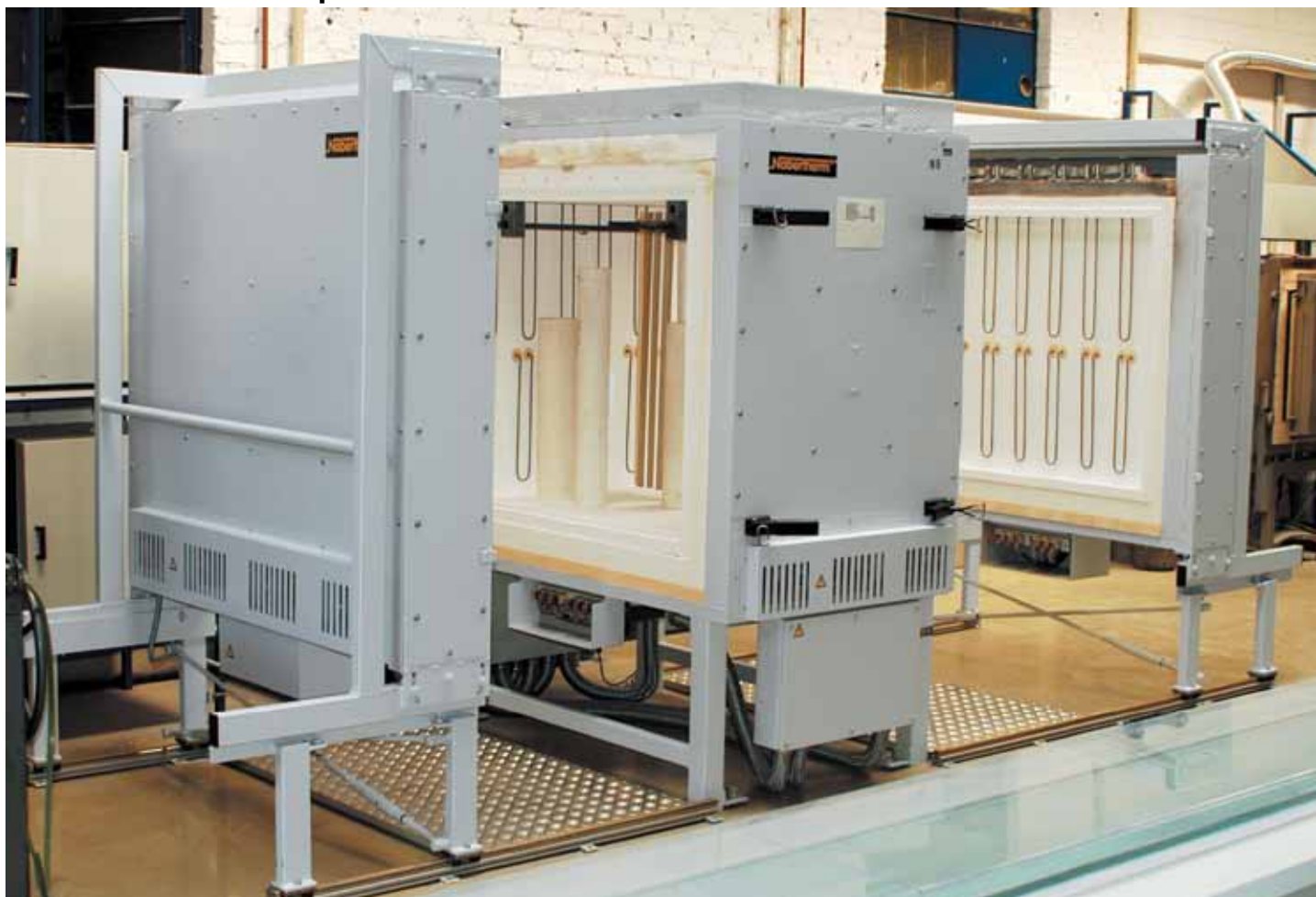
HT 1000/17 with two movable door segments and fourside heating for sintering hanging ceramic tubes up to 1700 °C
