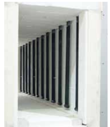
SiC rod elements on both sides of the furnace
