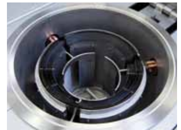
Cylindrical retort with tungsten heating
