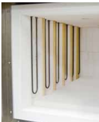
Protection of heating elements against mechanical damage
