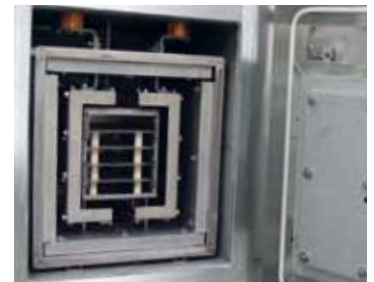
Molybdenum or tungsten heating chamber
