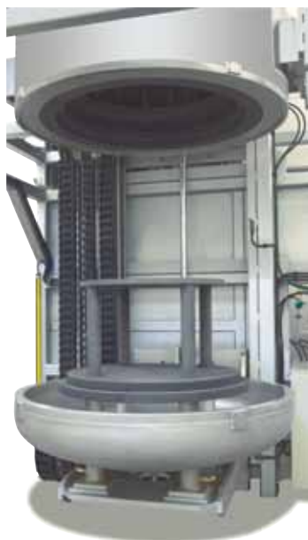
LBVHT with graphite heating chamber
