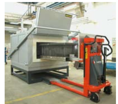
N 641 with annealing box and lift trolley
