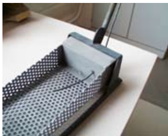
Thermocouple integrated in holder
