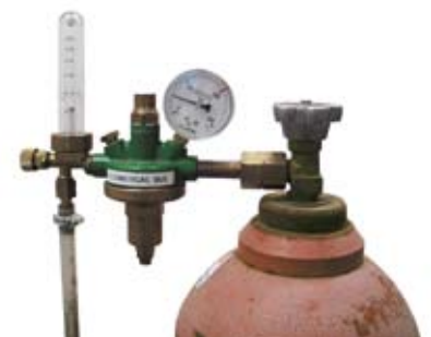
Pressure reducing valve with assembled flow meter
