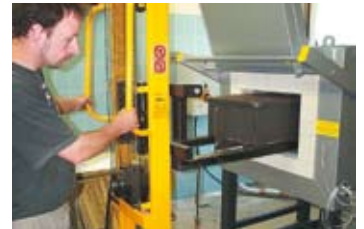
Winch stacker with hardening box and furnace
